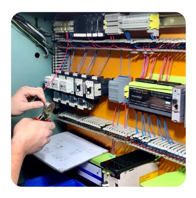
Our technicians begin by removing all the previous wiring and dated electronics from the machine in preparation for the new CNC set up. Once the new drives, contactors, heaters, communication switch, PLC, power supply, and the HMI touch screen have been mounted into place, everything can be wired up. The technicians will then calibrate the machine and test grind extensively before sending it back out for 30 more years of grinding.
