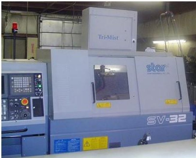
Direct Mount on Swiss lathe
